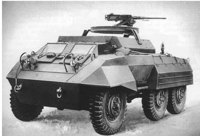
The M-20 Armored Utility Car mounted with a .50 caliber machine gun and command radios used by Tank Destroyer units as a command car.
