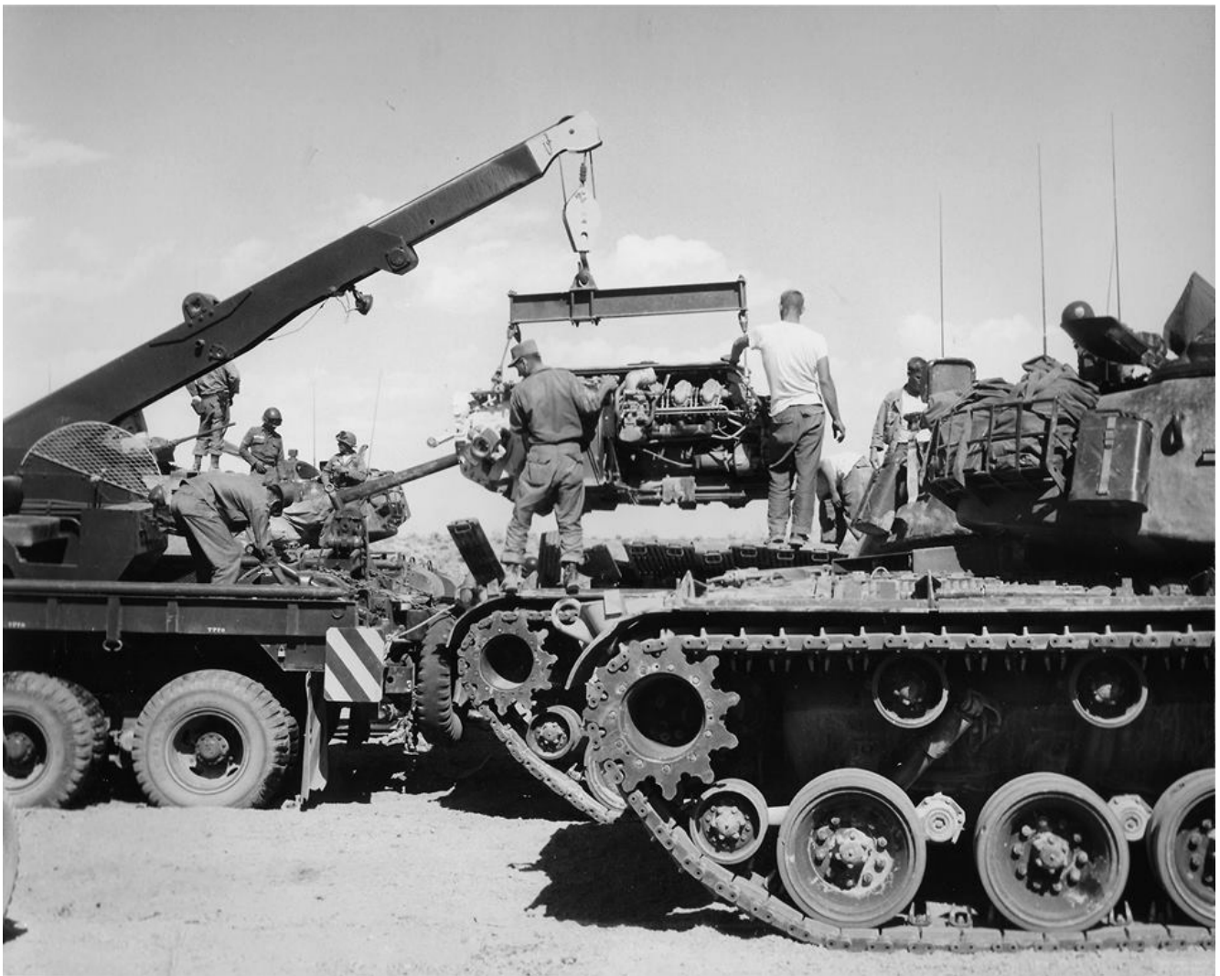
Soldiers from the 2nd Direct Support (DS) Platoon, 3632nd Ordnance Company removing an engine pack from an M48-series medium tank at the CON-SITE in 1961.
