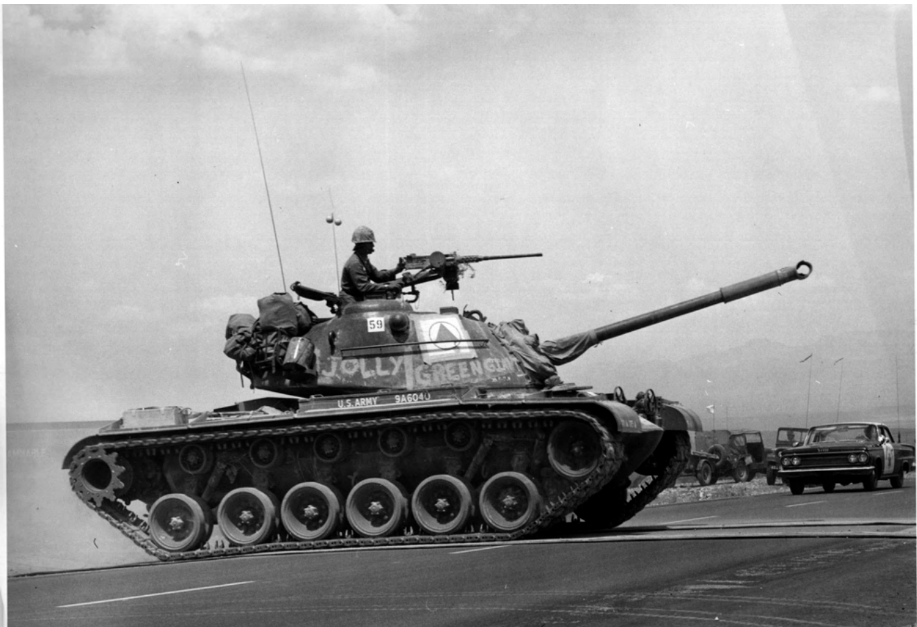
California Highway Patrol blocks traffic to allow a M48A1 tank of the 185th Armor to across a highway on rubber strips laid down to protect the pavement of the highway.
